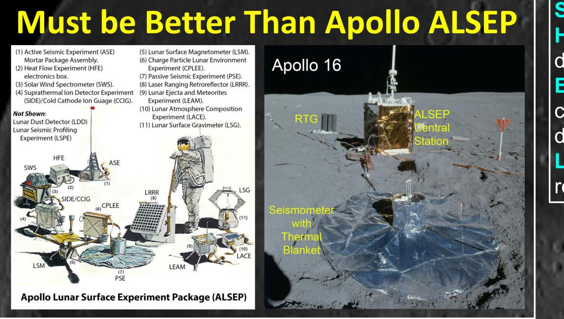
Lunar Science: Heat flow probes yield crustal heat budget estimates. Combined with EMS, the temperature profile of the deep interior can be modeled along with mineralogy. The seismic and LLR data also yield structure and compositional information of the lunar interior and the high fidelity data would enhance the usefulness of the GRAIL and Selene gravity data.
