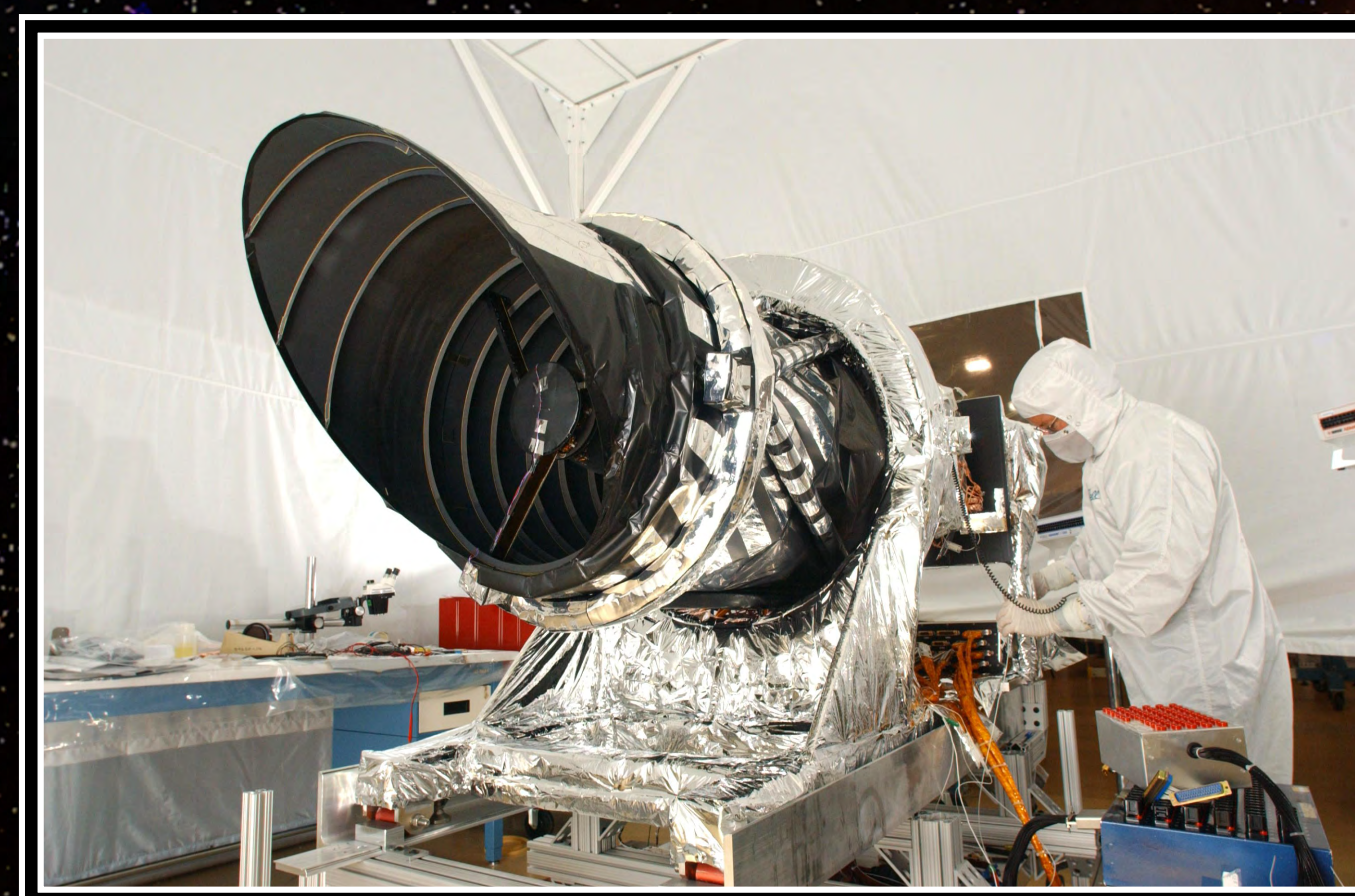
Figure 3: MRO/HIRISE's 0.5 m diameter mirror (shown here) and the 0.30 m diameter telescope on Deep Impact/EPOXI's High Resolution Imager (HRI) are two of the largest telescopes flown on planetary missions, for examples. In 2013 McEwen presented a "Mars Orbiting Space Telescope (MOST): Advancing Planetary Science (+Astrophysics, Heliophysics), Space Technology, and Human Spaceflight" concept for using the Hubble-class 2.4 m diameter telescopes provided to NASA by NRO [4]; McEwen similarly identified the ideal use of this telescope at Mars for optical communications technology demonstration.
