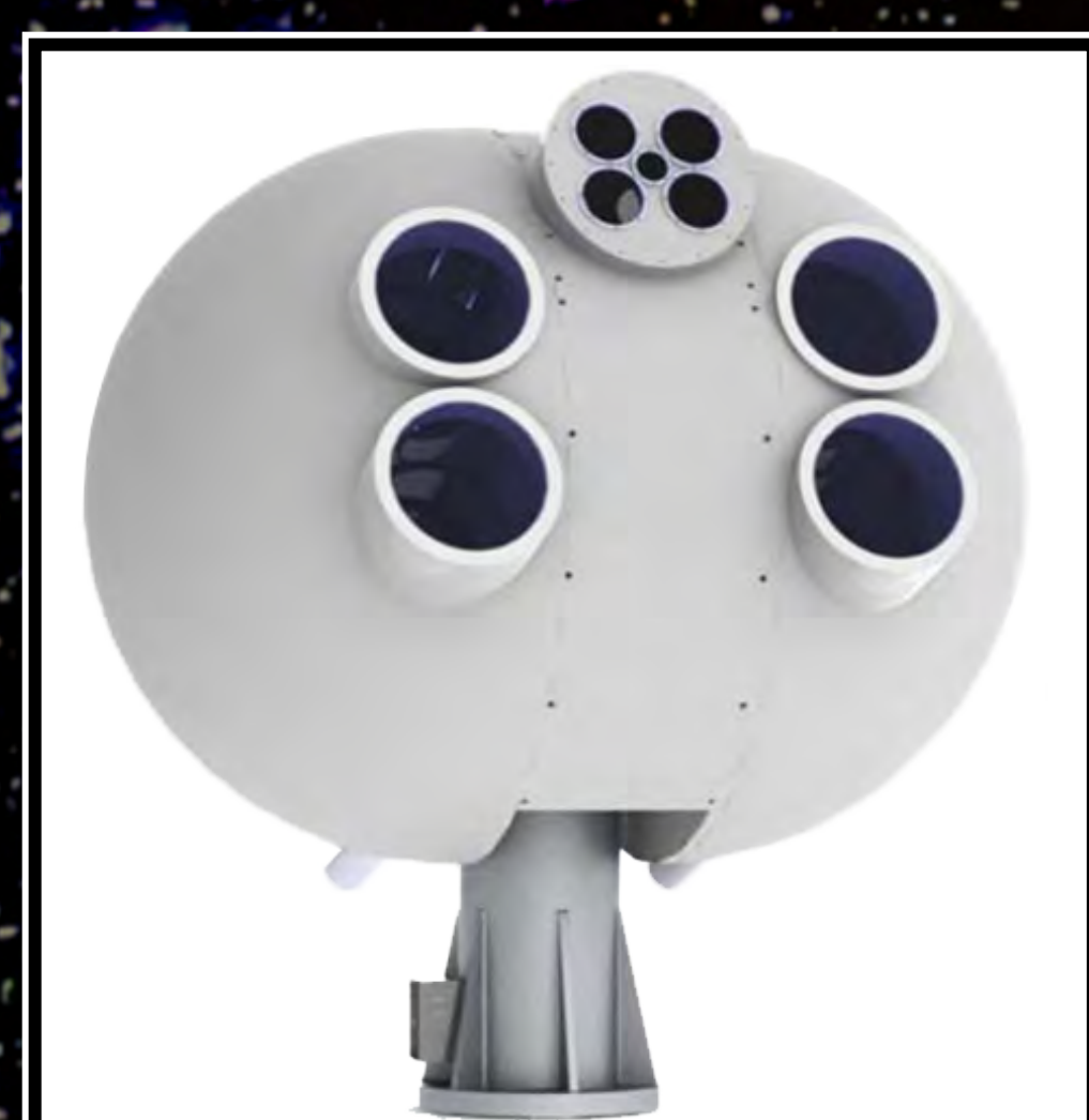
Figure 1: The LADEE Lunar Laser Communication Demonstration (LLCD) [3] achieved long-range uplinks at 10 and 20 Mbps, with downlinks in the 39 Mbps to 622 Mbps (top). A 0.10 m reflective telescope is coupled by optical fibers to a modern transmitter (bottom left). Its primary ground station terminal, located at White Sands, NM, was composed of four 40-cm telescopes for downlink and four 15-cm telescopes for uplink (bottom right). Alternate sites were located at NASA/JPL and ESA's OGS telescope in Tenerife, Spain. The successful demonstration of key technologies such as pointing, acquisition, and tracking from lunar orbit enables the progression of demonstrations at further distances on upcoming missions throughout the solar system in the next decades.
