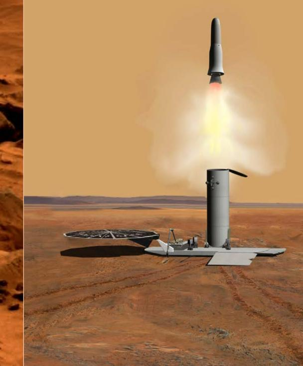
An artist's concept of a proposed Mars sample return mission [9; created in 2011], that portrays the launch of an ascent vehicle. The solar panels in the foreground are part of the rover that delivered the samples to the ascent vehicle.
